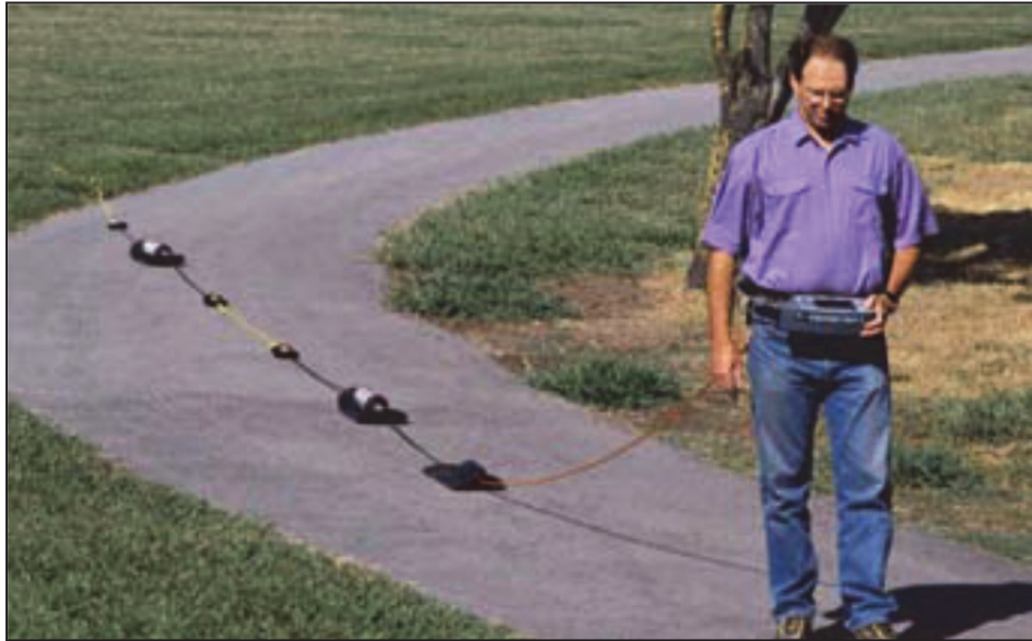
Figure 3.1—Towed Electrical Resistivity (ER) Array
