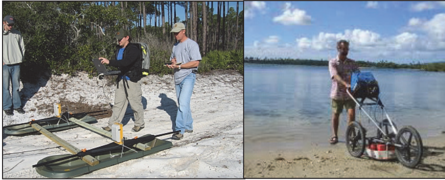
Figure 2.4—Representative Skid-mounted GPR and Wheeled Configurations
