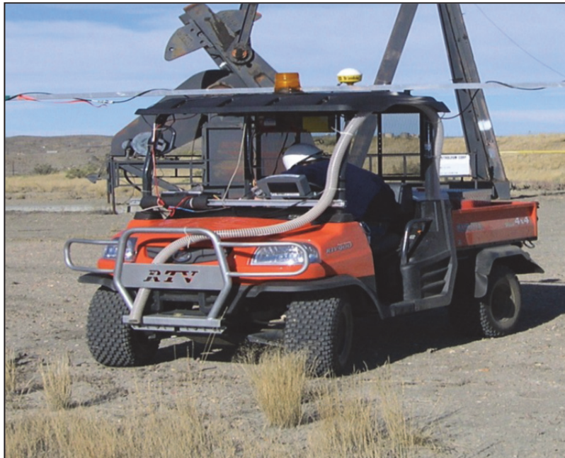
Figure 2.2—Mobile Gas Detector Mounted on ATV (Apogee Scientific)
